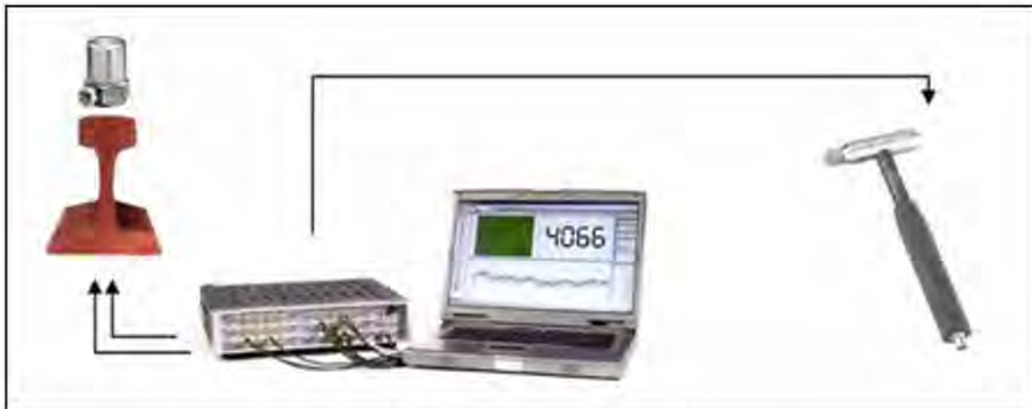
Figure 2.2 Measuring scheme for track decay rate.
