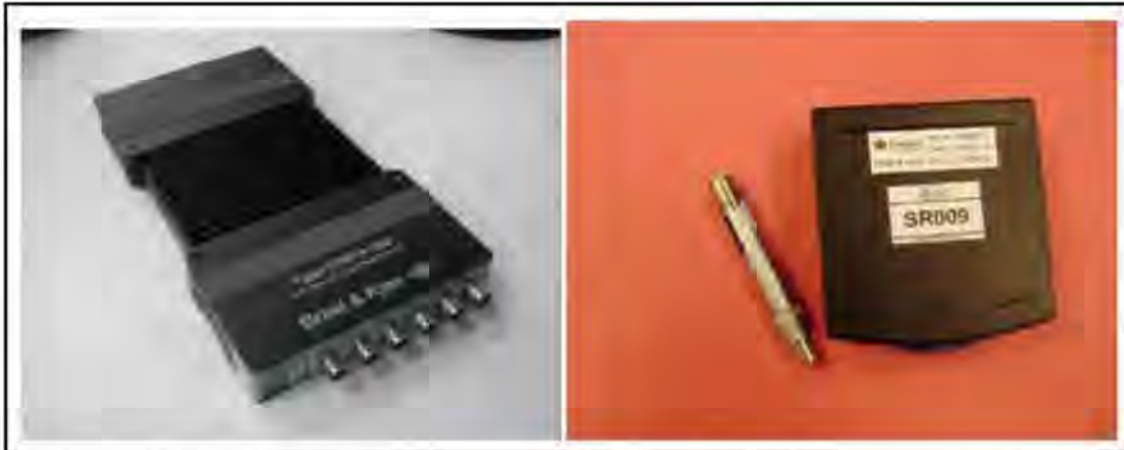
Figure 2.1 Record equipment 3050 LAN-XI and 1/2" microphone.
